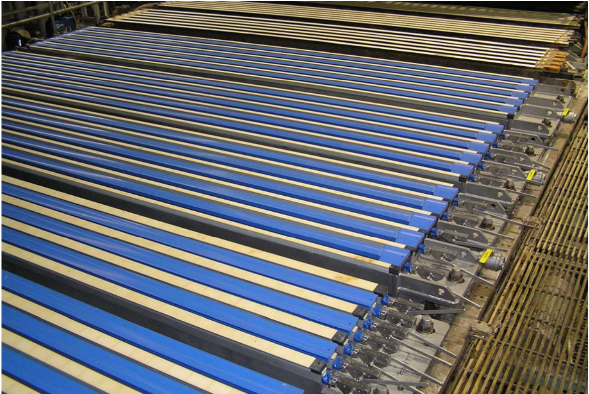
The addition of six table elements, and other proprietary operational changes, have increased the speed of the number one papermachine by 100 feet per minute.
